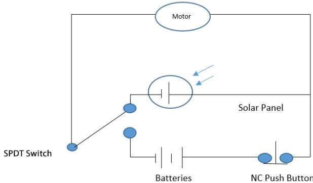
10. Each vehicle must include a mounted battery holder that is capable of holding two AA batteries. This system needs a switch and button as illustrated. This is to be used at the starting line as follows:
